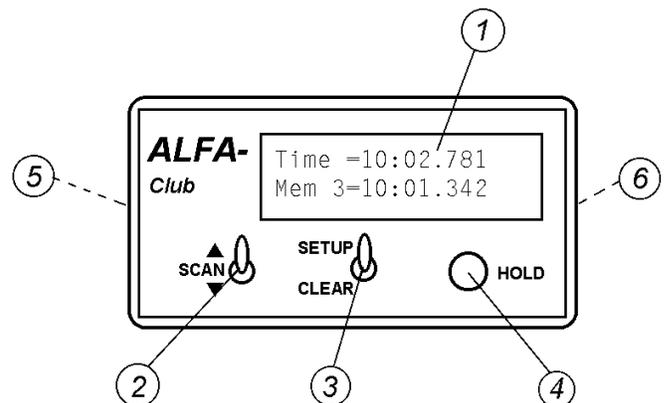
1. The **LCD** display shows the user all time, distance and memory information. It is also used to create interactive menus to configure the clock for use. While both the **ALFA-Club** and the **ALFA-**
