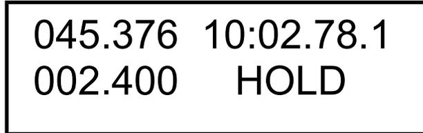
In Odometer Mode, pressing the HOLD button will alternately freeze and release the time and distance on the display. These continue to progress unseen, and the up to date values are displayed as soon as the Hold is released. The word “HOLD” appears in the lower right corner to remind you that the display is frozen. Note that the hold time is stored in the memory even when using Odometer Mode, and you may switch modes and review the memory at any time without effecting the odometer or the clock.
